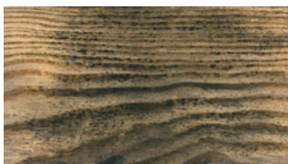
Mold infestation on spruce after one year of external weathering in a moist climate
